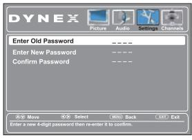
**6** Press the number buttons to enter the old password, then enter a new password. On the next line, enter the new password again to confirm it. The *Parental Controls* menu opens again.
